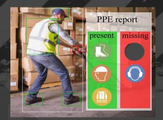
The objective is to develop algorithms for the detection of two common workplace injuries precursors: 1) non-use of personal protective equipment and 2) nonergonomic execution of repetitive work assignments.
